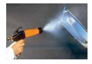
Super Vortex round spray: The narrow pattern (1) is to force paint into hollow parts and cavities, the wider pattern (3) is to spray as fast as possible with the best wrap possible.
