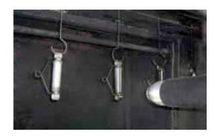
For the parts to attract the paint drops, they and whatever they are hanging from must be properly grounded. An uninterrupted connection must be established from the part throughout the rack, the hook, the rotator to the conveyor, which is grounded by construction.
