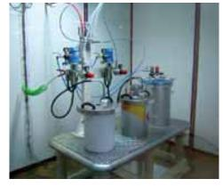
Water-borne paint supply, isolated of the ground potential, dedicated to electrostatic application with internal electrostatic charge.
